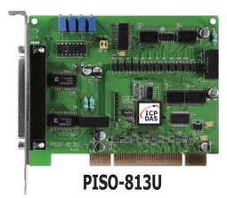
Universal PCI, 10 kS/s, 32-ch, 12-bit Isolated Analog Input **Board**
